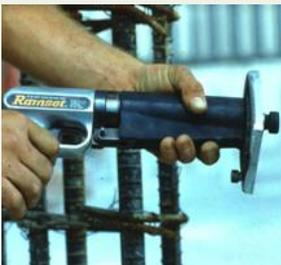
Powder-actuated tools should never be stored or used in explosive atmospheres, or in the vicinity of highly flammable materials, or anywhere non-sparking tools are required.
